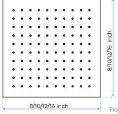
1/2" NPT inlets Easy clean nozzles Flow Rate: 9.5L/min 2.5 GPM
